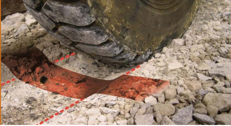
Rutting accumulation at the surface and the subgrade were used to compare geogrid performance.
