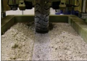
Trafficking of Tensar ® BX Geogrid
