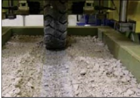
Trafficking of Tensar TriAx Geogrid
