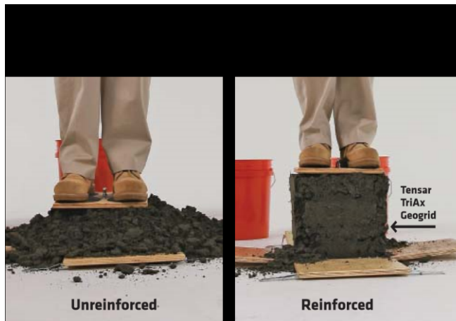
FIGURE 1 The lateral confinement of aggregate reinforcement with Tensar TriAx Geogrid is demonstrated through the box of rocks demonstration.
